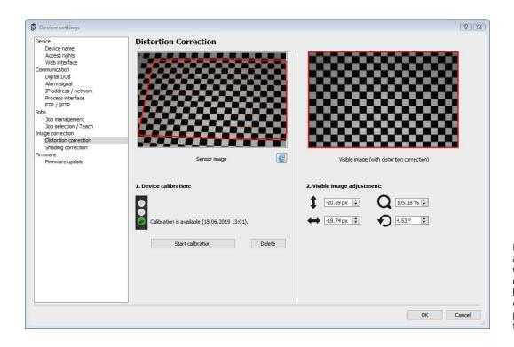
Image distortions can be automatically corrected and world coordinates configured in *Application Suite* by mouse click using the calibration plate, which is placed in the visible area of the vision sensor.
