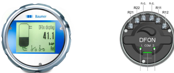
Figure 9: Example of sensor electronics with two optoelectronic relay contacts
