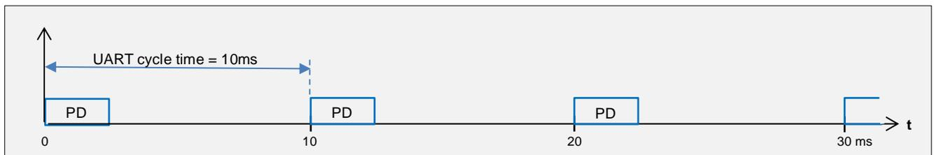
Diagram 1: Transmission of the process data (PD) from MSP to STM32.
